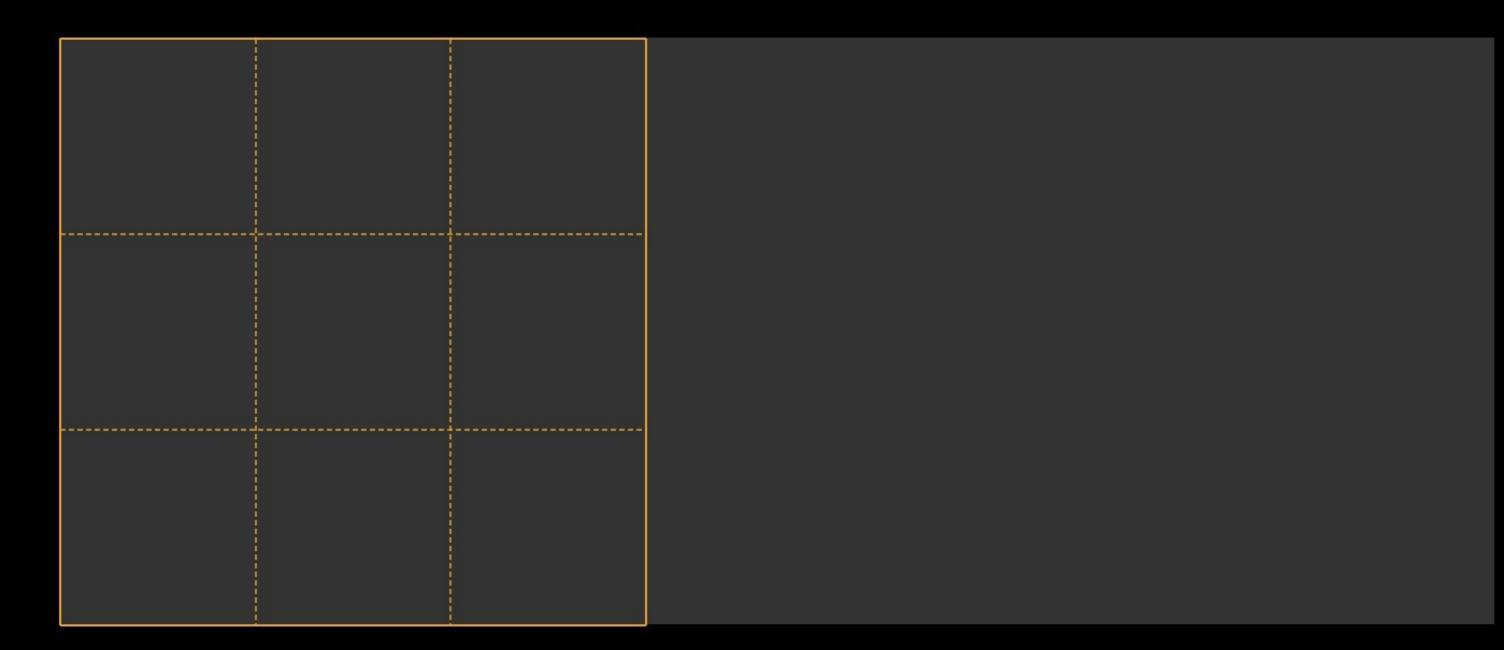
Build the grid with tracks using grid-template-columns & grid-template-rows
